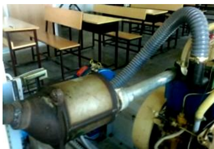
FIGURE 4: ENGINE SETUP WITH CATALYTIC CONVERTER
